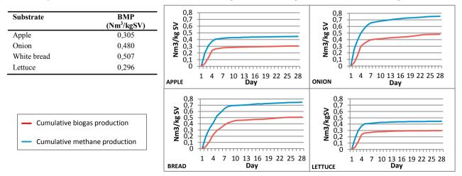
Fig. 4. Methane yields in BMP tests and cumulative biogas and methane production
